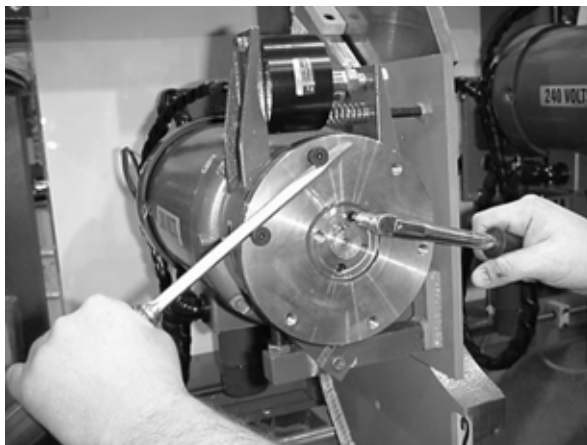
Figure 3: Hold the Hub Still While Adjusting the Bushing Screws
